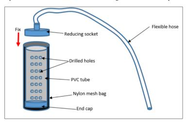
Figure 3. Diagrammatic representation of the siphoning device
